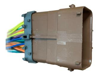
B—**C-36 Connector:** The brown in-line connector plugs into the main control pack harness. This will provide the necessary power signals needed for engine operation.
